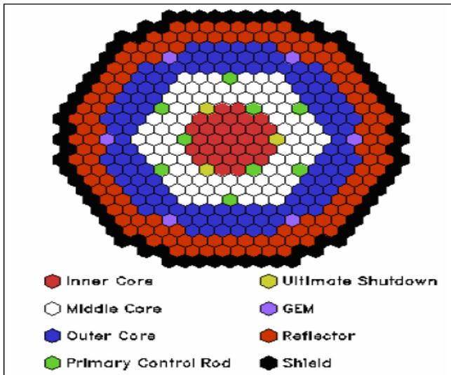
Figure 1.4 Reference Design Core Layout
