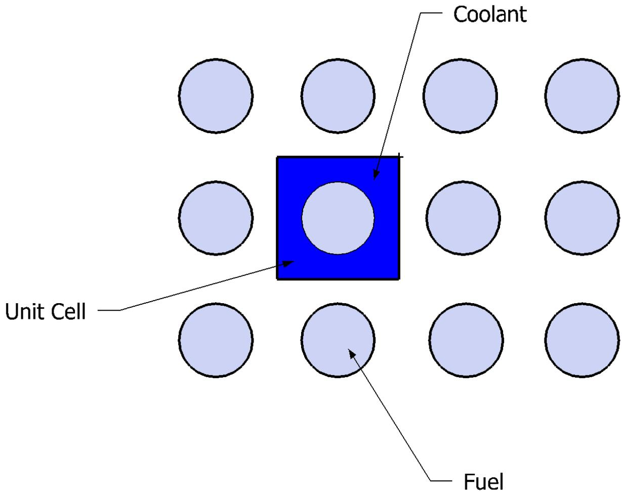
Figure 1.1 A square Unit Cell For a Pin cell Core
