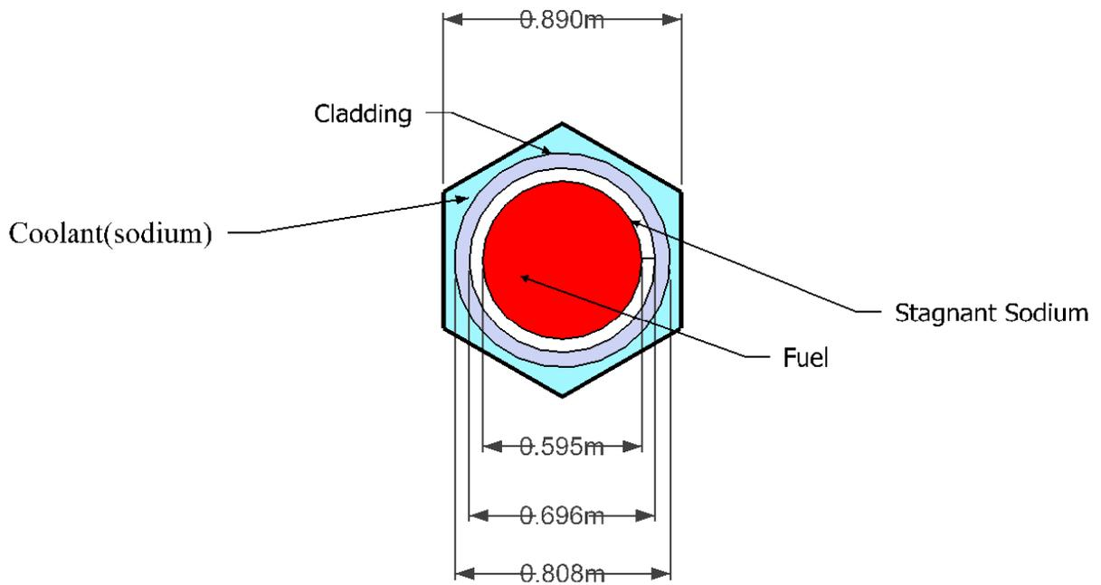
Figure 1.5 A unit cell of reference pin cell
