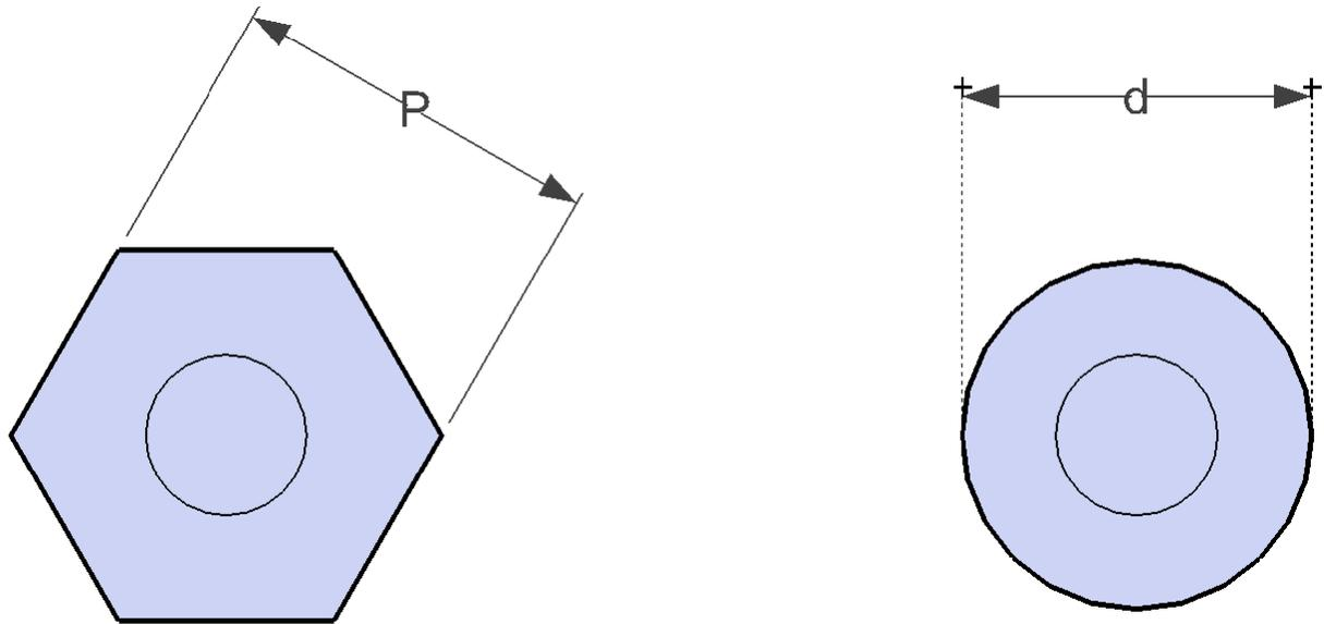
Figure 1.3 The Concept of an Equivalent Diameter
