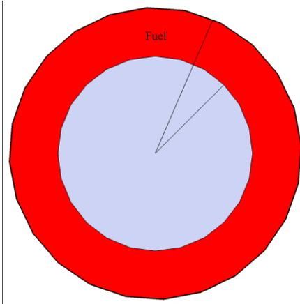
Figure 2.0 A TID Equivalent Cell After smearing
