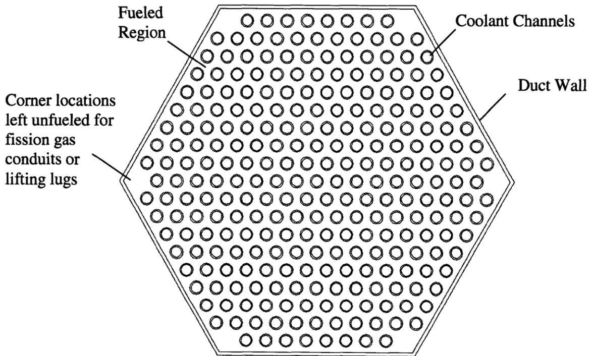
Figure 1.2 A Hexagonal TID Assembly
