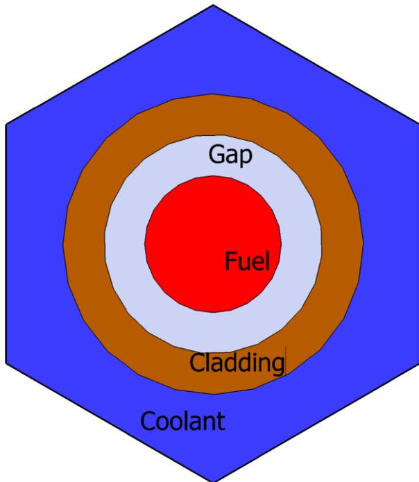
Figure 1.6 Reference pin cell Before Smearing
