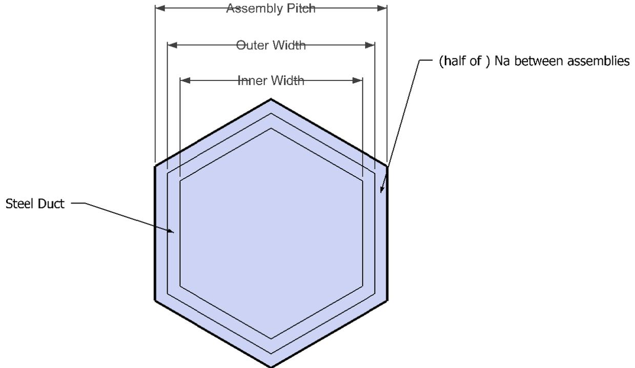
Figure 2.3 Cross section of a hexagonal assembly
