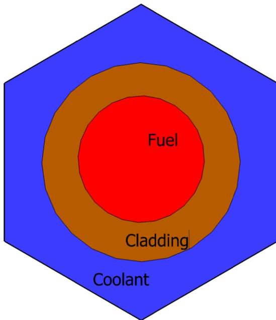
Figure 1.7 Reference pin cell After Smearing
