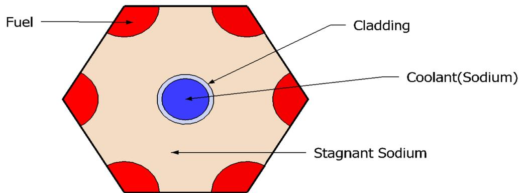
Figure 1.8 A TID Unit Cell
