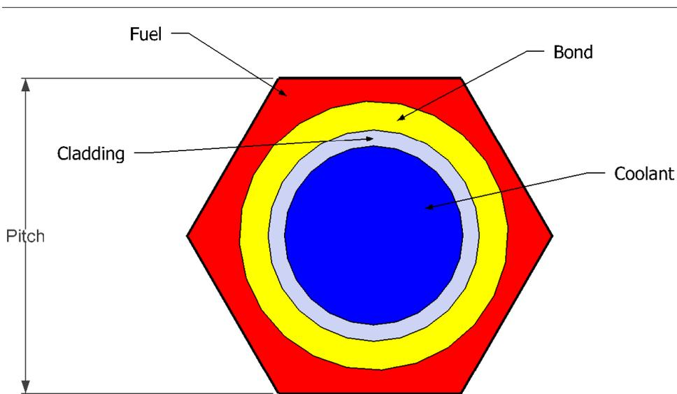
Figure 2.8 NOVEX 1.2 Design before smearing
