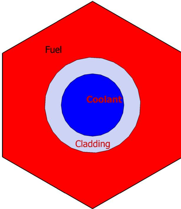
Figure 1.9 TID unit cell after smearing
